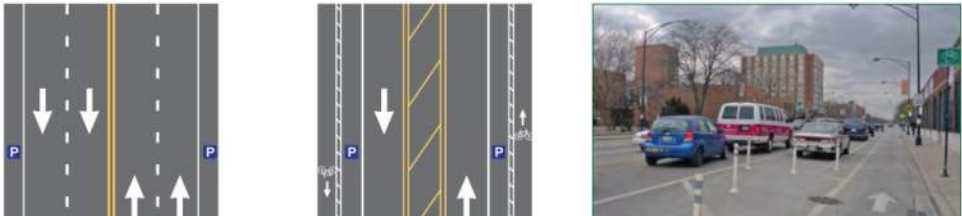
Figure 2. Chicago, Illinois – 55th Street. FHWA case-study graphic showing the conversion from a 4-lane street to a 3-lane street with parking-separated bicycle lanes. Source: FHWA Road Diet Case Studies, pp. 9–10.
