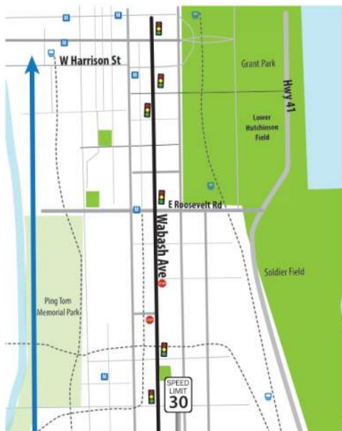
Figure 3. Chicago, Illinois – Wabash Avenue. FHWA case-study graphic showing a 4-to-3 conversion with buffered bike lanes and signal optimization. Source: FHWA Road Diet Case Studies, pp. 13–14.
