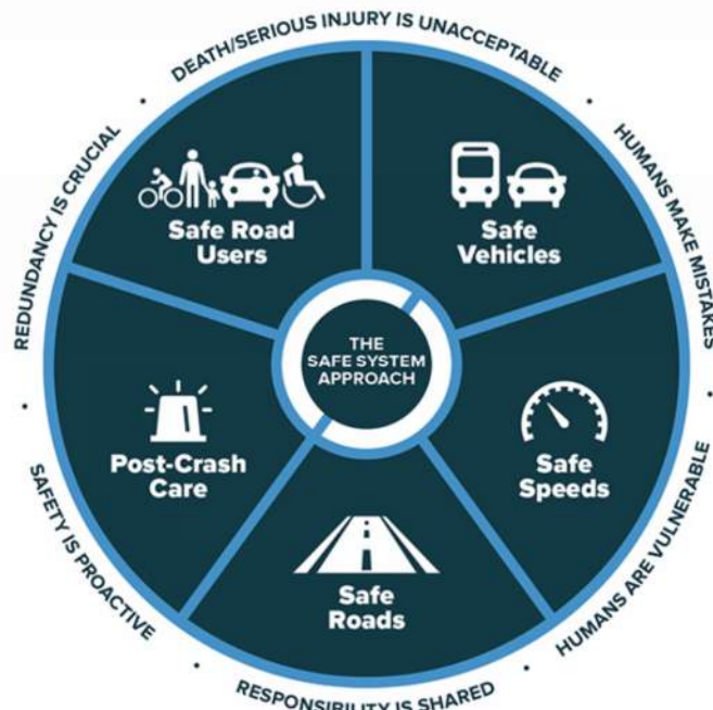
Figure 1 - Safe System Approach
